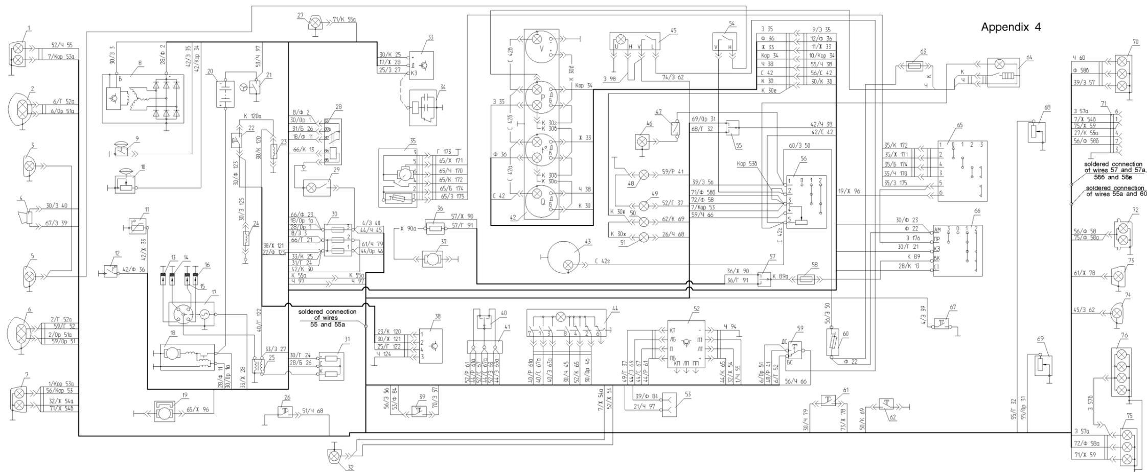
Fig. 1. Wiring Diagram of Automobile YA3-31512:
